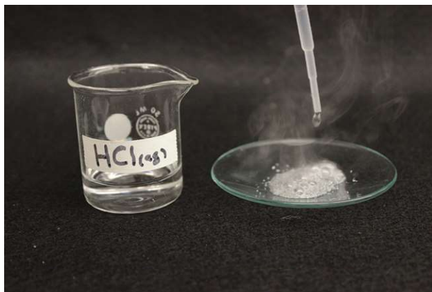
Figure 18.27 The reaction of iron with an acid produces hydrogen. Here, iron reacts with hydrochloric acid. (credit: Mark Ott)
