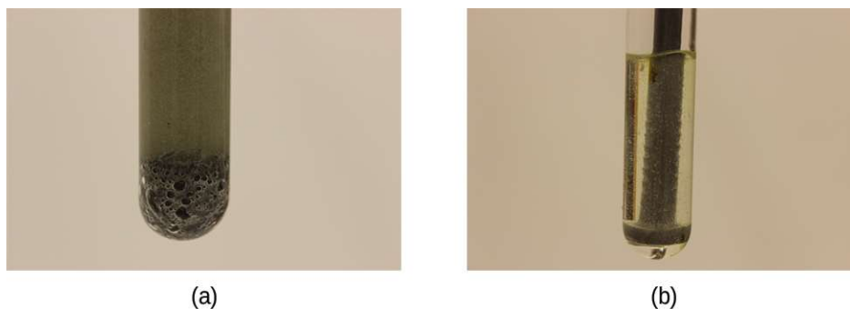
Figure 17.6 (a) Iron powder reacts rapidly with dilute hydrochloric acid and produces bubbles of hydrogen gas: 2\text{Fe}(s) + 6\text{HCl}(aq) \rightarrow 2\text{FeCl}_3(aq) + 3\text{H}_2(g) . (b) An iron nail reacts more slowly because the surface area exposed to the acid is much less.
