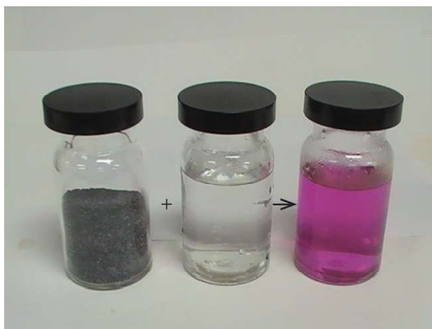
Figure 18.6 From left to right: Mg(s), warm water at pH 7, and the resulting solution with a pH greater than 7, as indicated by the pink color of the phenolphthalein indicator. (credit: modification of work by Sahar Atwa)
