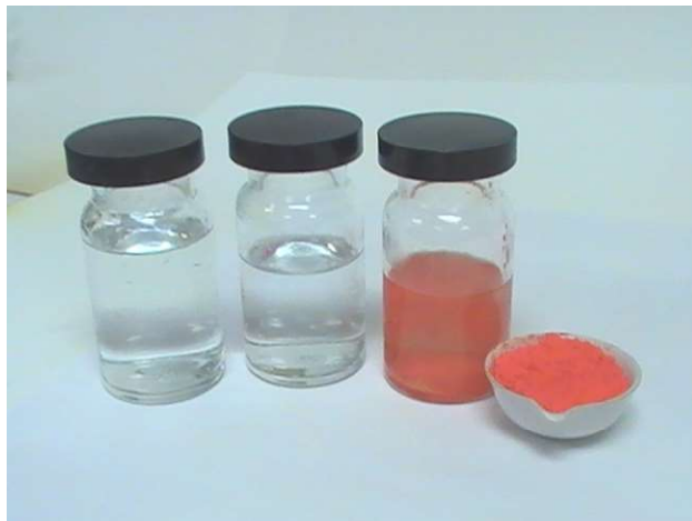
Figure 18.61 Solid \text{HgI}_2 forms when solutions of \text{KI} and \text{Hg}(\text{NO}_3)_2 are mixed. (credit: Sahar Atwa)
