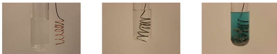
Figure 16.2 A copper wire and an aqueous solution of silver nitrate (left) are brought into contact (center) and a spontaneous transfer of electrons occurs, creating blue \text{Cu}^{2+}(aq) and gray \text{Ag}(s) (right).
