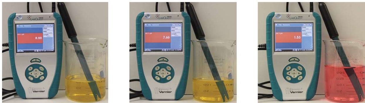
Figure 14.16 The indicator color (methyl orange) shows that a small amount of acid added to a buffered solution of pH 8 (beaker on the left) has little effect on the buffered system (middle beaker). However, a large amount of acid exhausts the buffering capacity of the solution and the pH changes dramatically (beaker on the right). (credit: modification of work by Mark Ott)
