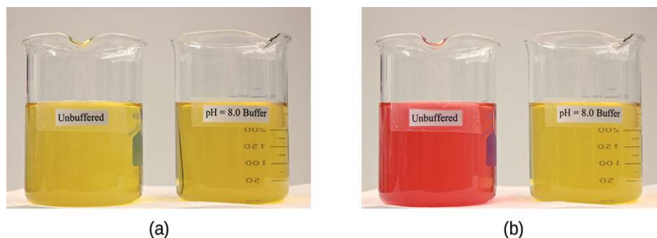
Figure 14.14 (a) The buffered solution on the left and the unbuffered solution on the right have the same pH (pH 8); they are basic, showing the yellow color of the indicator methyl orange at this pH. (b) After the addition of 1 mL of a 0.01- M HCl solution, the buffered solution has not detectably changed its pH but the unbuffered solution has become acidic, as indicated by the change in color of the methyl orange, which turns red at a pH of about 4. (credit: modification of work by Mark Ott)
