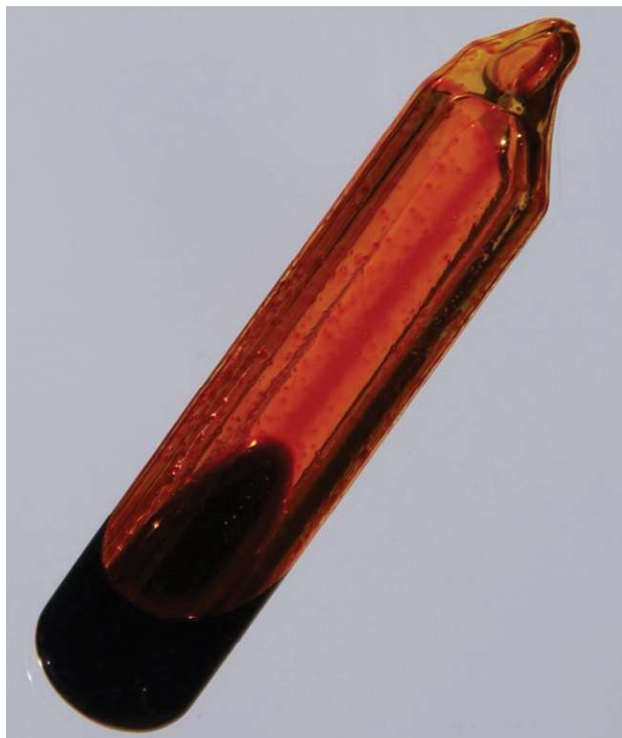
Figure 13.4 A sealed tube containing an equilibrium mixture of liquid and gaseous bromine. (credit: http://images-of-elements.com/bromine.php )
