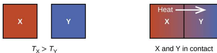
Figure 12.5 When two objects at different temperatures come in contact, heat spontaneously flows from the hotter to the colder object.
