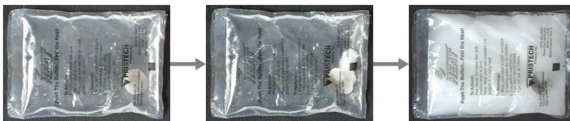
Figure 11.17 This hand warmer produces heat when the sodium acetate in a supersaturated solution precipitates. Precipitation of the solute is initiated by a mechanical shockwave generated when the flexible metal disk within the solution is “clicked.” (credit: modification of work by “Velela”/Wikimedia Commons)
