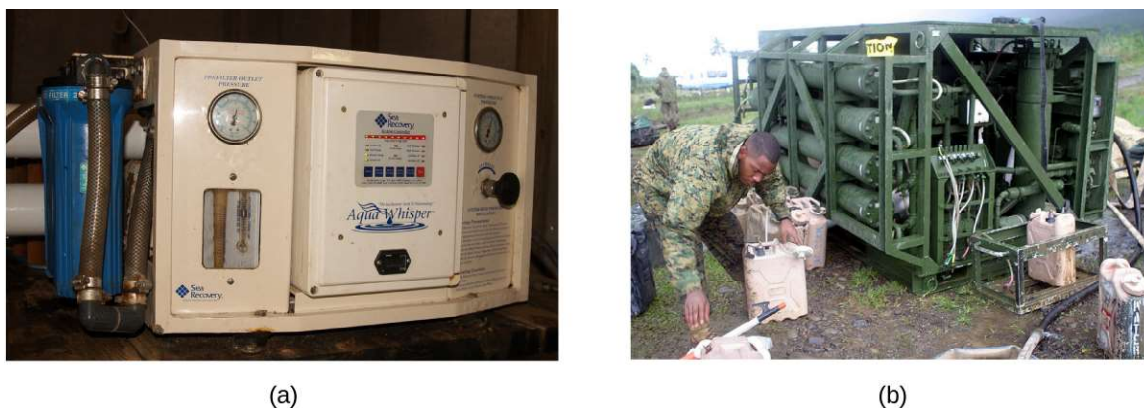
Figure 11.26 Reverse osmosis systems for purifying drinking water are shown here on (a) small and (b) large scales. (credit a: modification of work by Jerry Kirkhart; credit b: modification of work by Willard J. Lathrop)
