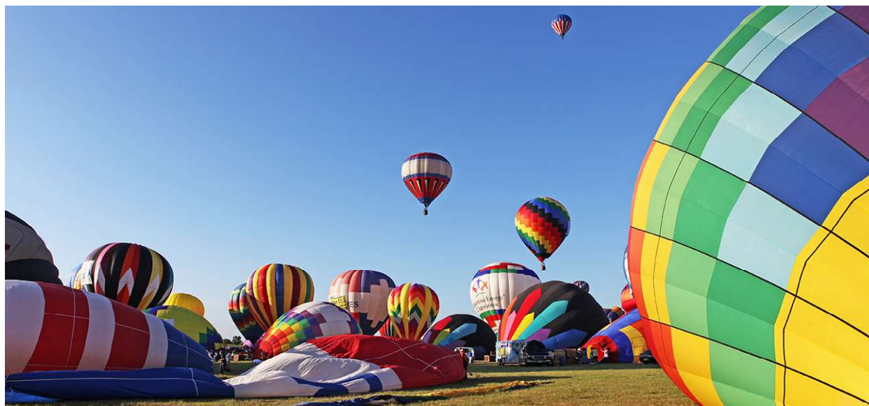
Figure 8.1 The hot air inside these balloons is less dense than the surrounding cool air. This results in a buoyant force that causes the balloons to rise when their guy lines are untied. (credit: modification of work by Anthony Quintano)
