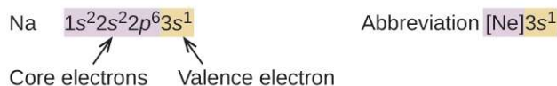
Figure 3.28 A core-abbreviated electron configuration (right) replaces the core electrons with the noble gas symbol whose configuration matches the core electron configuration of the other element.
