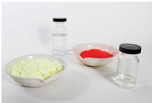
Figure 2.26 Each sample contains 6.02 \times 10^{23} molecules or formula units—1.00 mol of the compound or element. Clockwise from the upper left: 130.2 g of \text{C}_8\text{H}_{17}\text{OH} (1-octanol, formula mass 130.2 amu), 454.4 g of \text{HgI}_2 (mercury(II) iodide, formula mass 454.4 amu), 32.0 g of \text{CH}_3\text{OH} (methanol, formula mass 32.0 amu) and 256.5 g of \text{S}_8 (sulfur, formula mass 256.5 amu). (credit: Sahar Atwa)
