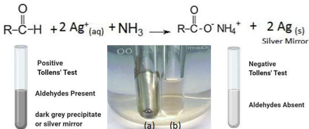
Figure 25.5: (a) Positive Tollens Test (b) Negative Tollens Test. credit: author modified, https://en.wikipedia.org/wiki/Tollens
