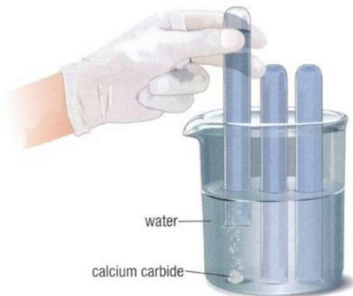
Figure 23.4: Experimental setup for collecting acetylene gas. credit: http://fon10.weebly.com/uploads/1/3/4/7/13472506/2_5_activity_ethynecombustion.pdf
