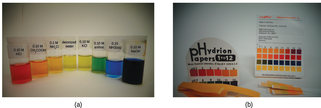
Figure 3.34 (a) A universal indicator assumes a different color in solutions of different pH values. Thus, it can be added to a solution to determine the pH of the solution. The eight vials each contain a universal indicator and 0.1-M solutions of progressively weaker acids: HCl (pH = 1), CH 3 CO 2 H (pH = 3), and NH 4 Cl (pH = 5), deionized water, a neutral substance (pH = 7); and 0.1-M solutions of the progressively stronger bases: KCl (pH = 7), aniline, C 6 H 5 NH 2 (pH = 9), NH 3 (pH = 11), and NaOH (pH = 13). (b) pH paper contains a mixture of indicators that give different colors in solutions of differing pH values. (credit: modification of work by Sahar Atwa)
