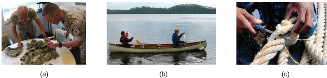
Figure 3.65 (a) These soldiers are sorting through pieces of a Kevlar helmet that helped absorb a grenade blast. Kevlar is also used to make (b) canoes and (c) marine mooring lines. (credit a: modification of work by "Cla68"/Wikimedia Commons; credit b: modification of work by "OakleyOriginals"/Flickr; credit c: modification of work by Casey H. Kyhl)
