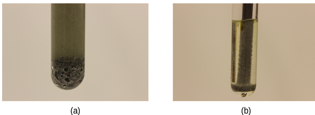
Figure 7.32 (a) Iron powder reacts rapidly with dilute hydrochloric acid and produces bubbles of hydrogen gas because the powder has a large total surface area: 2\text{Fe}(s) + 6\text{HCl}(aq) \longrightarrow 2\text{FeCl}_3(aq) + 3\text{H}_2(g) . (b) An iron nail reacts more slowly.
