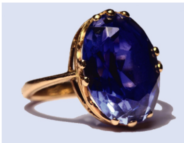
Figure 3.13 Although pure aluminum oxide is colorless, trace amounts of iron and titanium give blue sapphire its characteristic color. (credit: modification of work by Stanislav Doronenko)
