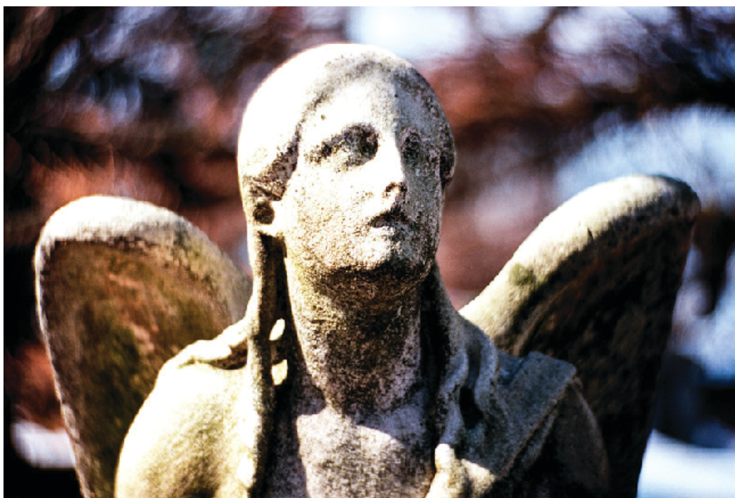
Figure 7.33 Statues made from carbonate compounds such as limestone and marble typically weather slowly over time due to the actions of water, and thermal expansion and contraction. However, pollutants like sulfur dioxide can accelerate weathering. As the concentration of air pollutants increases, deterioration of limestone occurs more rapidly. (credit: James P Fisher III)
