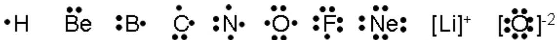
Figure 1.9 Lewis structure examples of the second row elements (Hydrogen to Neon), a cation (Lithium has lost its one valence electron), and an anion (Oxygen has gained two valence electrons). credit: author
