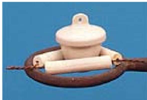
Figure 14.7: Setup for heating a crucible. Leave the cover ajar, to allow gas to escape but larger particles can not. credit: " The Composition of Potassium Chlorate (Experiment)" by Santa Monica College, LibreTexts is licensed under CC BY-NC .
