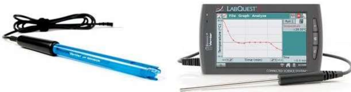
Figure 17.5: pH Probe and Lab Quest 2 from Vernier. credit: (a) https://www.vernier.com/files/manuals/gdx-ph-bnc/gdx-ph-bnc.pdf (b) https://www.vernier.com/product/labquest-2/
