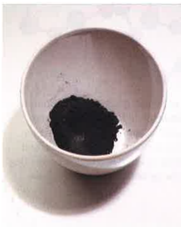
▲ Aluminum oxide crucible, a container in which substances can be subjected to high temperatures.
